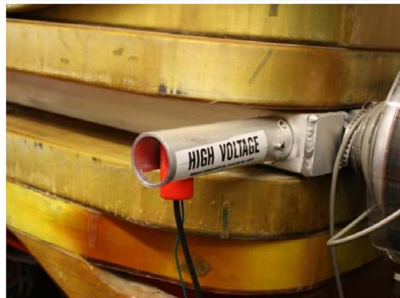
HV feedthroughs of ion pumps are most vulnerable, needing protection
