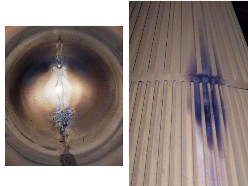
Electron beam melted through aluminum body
